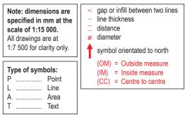
Most of the symbols in this specification shall be orientated to north. That a symbol is to be orientated to north is indicated with an arrow pointing upward beside the symbol. When a symbol shall be orientated to north, it means that it shall be orientated to magnetic north and hence relative to the edges of the paper and the magnetic north lines.
